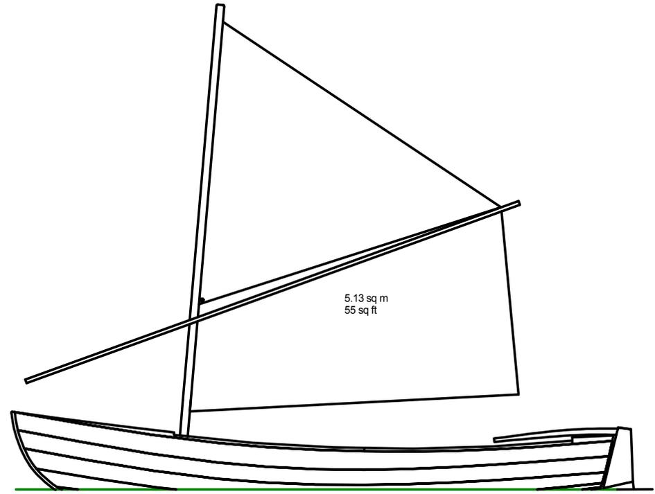
This drawing demonstrates the principle of "scandalizing" as a quick method of reefing. As you can see, the sprit is moved to a cringle on the leech positioned such that the head of the sail folds down neatly to be secured to the mast. This system can be used in addition (or as an alternative) to the conventional reefing shown on the sail-plan. Consult sailmaker.
