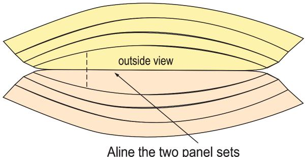
Aline the two panel sets and tape along the keel seam on the inside.
