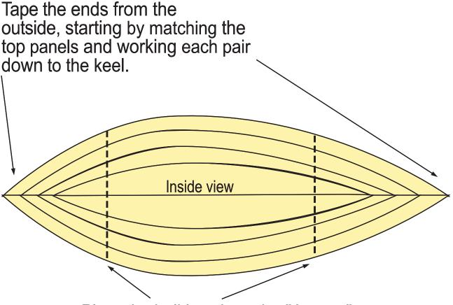
Place the bulkheads at the "Arrows" marked on the hull. The bulkheads are used to maintain hull shape to show the lines of the O&P Pod.
