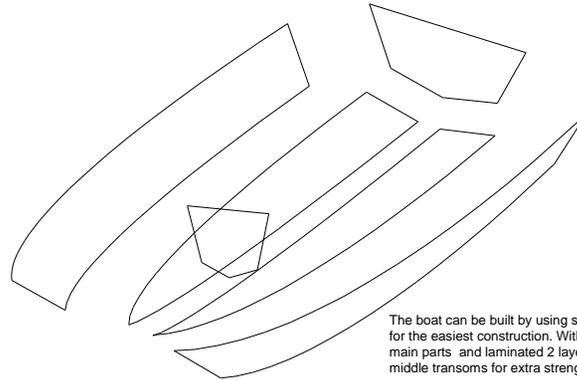
The boat can be built by using stitch and glue method for the easiest construction. With 6mm plywood for the main parts and laminated 2 layers of 6mm for the middle transoms for extra strength.
